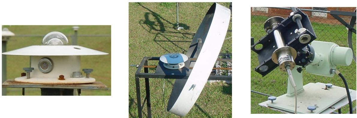
Fig.3: Global, diffuse and direct solar measuring devices.
